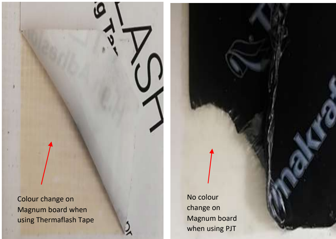
Figure 2. Peel adhesion test of Health Based Building Magnum boards
