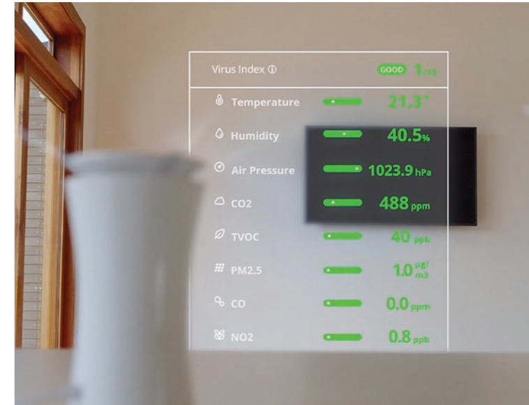
The uHoo data capture monitor from the Foreverbreathe Demonstration Home showing an ideal reading where all levels appear in green.
