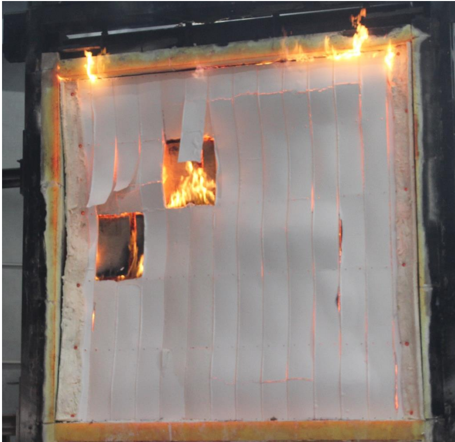
Figure 16 – Exposed face after the test
