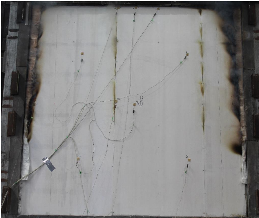
Figure 15 – Unexposed face at 90 minutes
