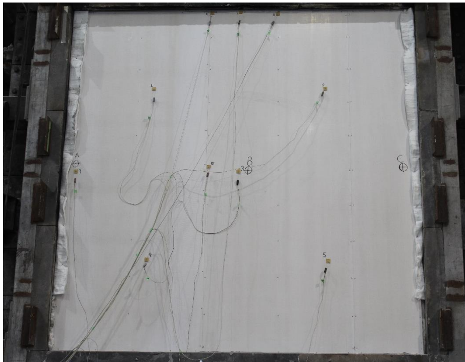
Figure 11 – Unexposed face prior to test commencement
