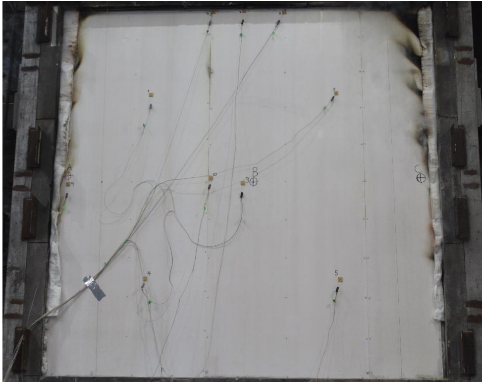
Figure 14 – Unexposed face at 60 minutes
