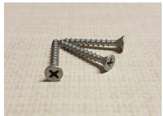
Fortress Fasteners 6g x 32mm C3 Galvanised Collated Screws Individual code FCS632CL3J for fixing Magnum Board to timber framing
