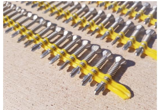
Simpson Strong Tie 8g x 32mm C3 Galvanised Wing Tip Collated Square Drive Screws code CBSDG114SA for fixing Magnum Board to steel framing
