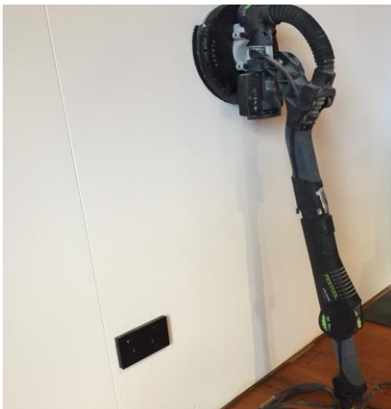
Recommended mechanical sanding equipment
