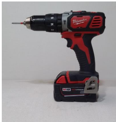
Battery powered drill gun with torque controller
