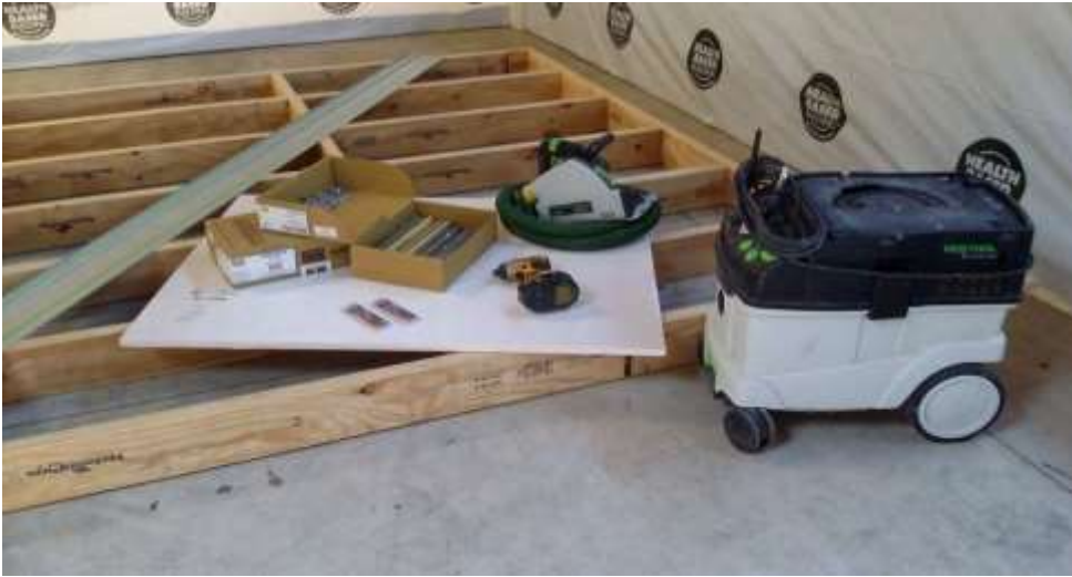
HEPA extraction system with recommended cutting equipment
