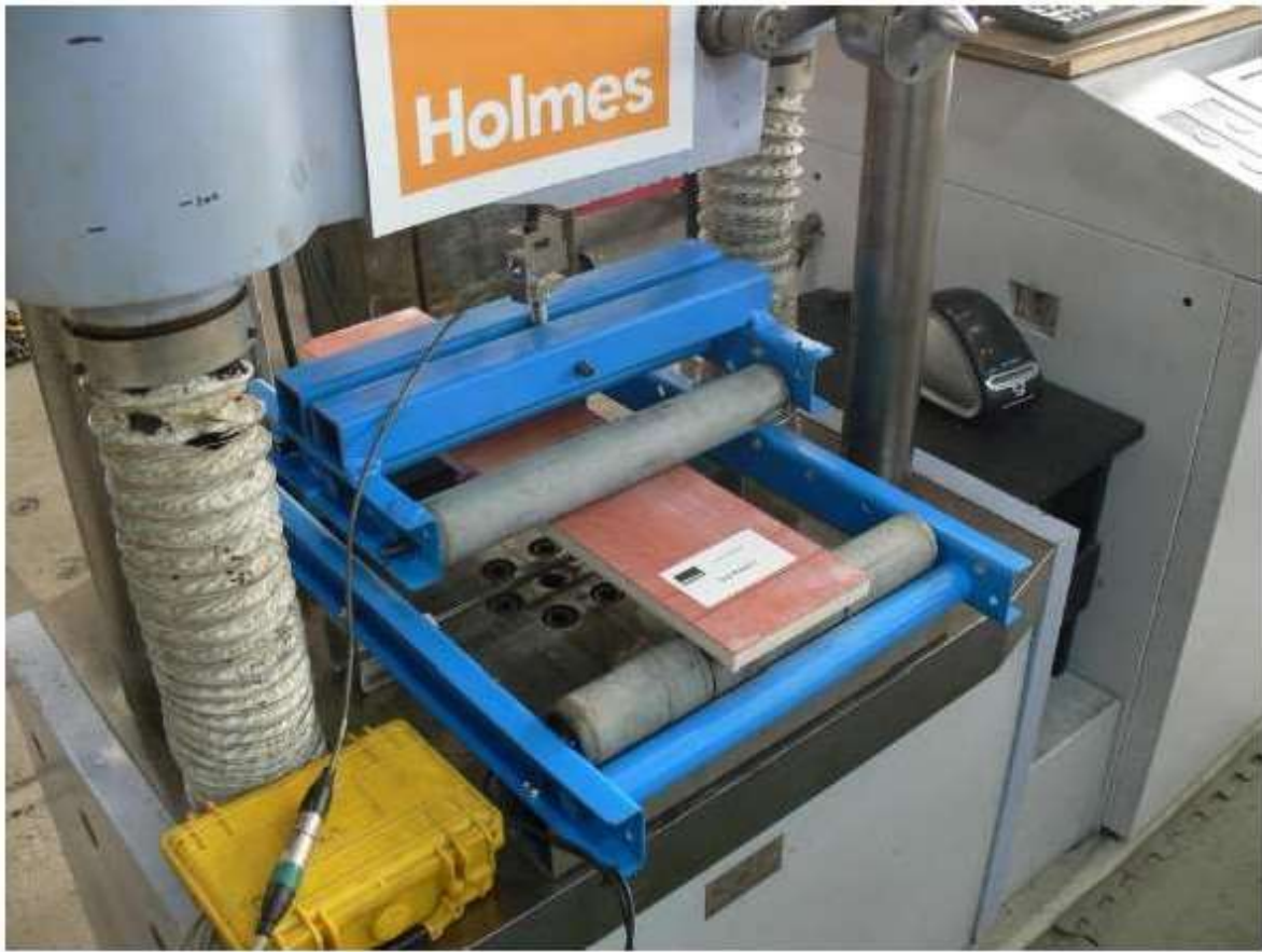
Figure 1: Four Point Bend Apparatus and test sample
