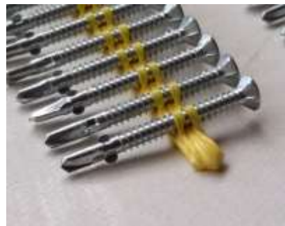
Simpson Strong Tie screw for steel framing code: SSBFHSD2SA 10-gauge x 50mm #2 Square Drive Wing Tip Stainless Steel 316
