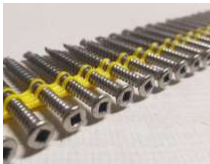
Simpson Strong Tie screw for timber framing code: SSDHSD50TSA 10-gauge x 50mm #2 Square Drive Pre-Bore Tip Stainless Steel 305
